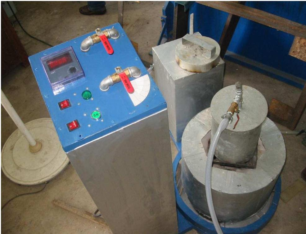
Fig. 13. A low-cost machine for countergravity casting
