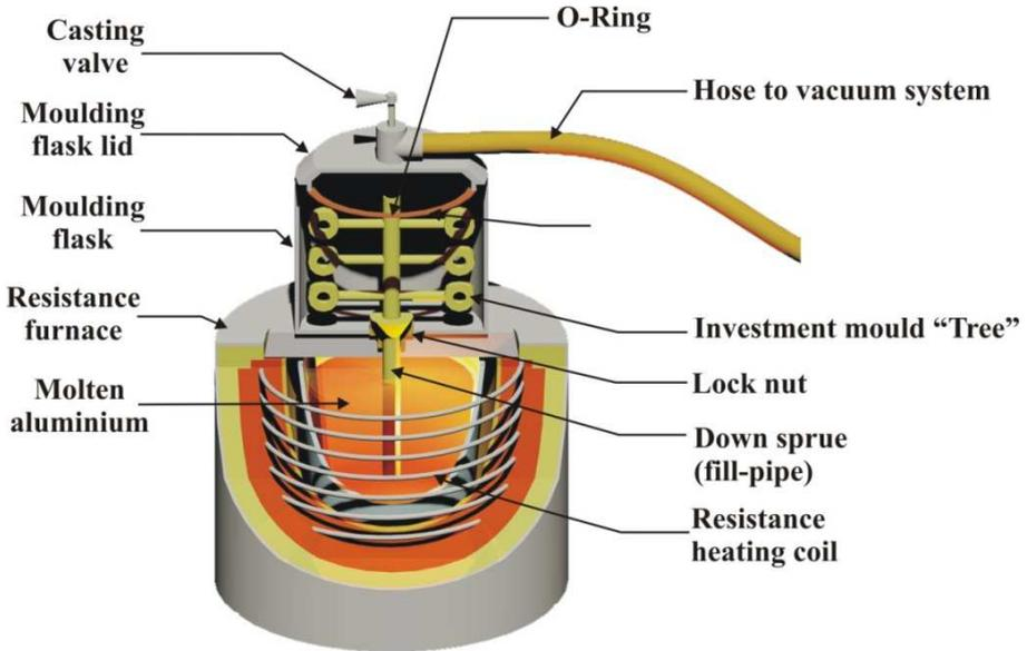
Fig. 1. Typical setup of the countergravity casting process
