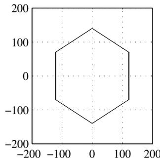
Fig. 4. Hexagon of feasible filter current.
