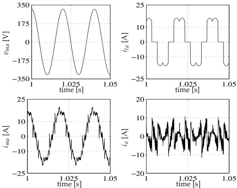
Fig. 11. Current and line voltage waveforms on phase *a*: diode bridge load scenario.
