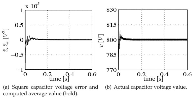
Fig. 9. Voltage controller performance: two harmonics load scenario.
