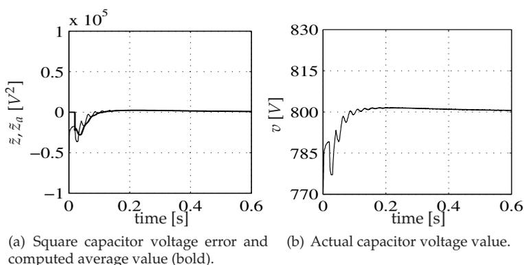
Fig. 13. Voltage controller performance: diode bridge load scenario.
