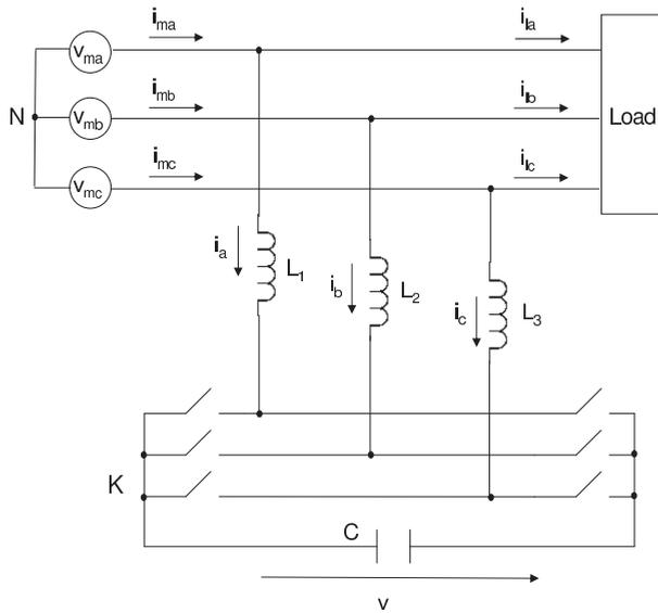
Fig. 1. Shunt Active Filter scheme.
