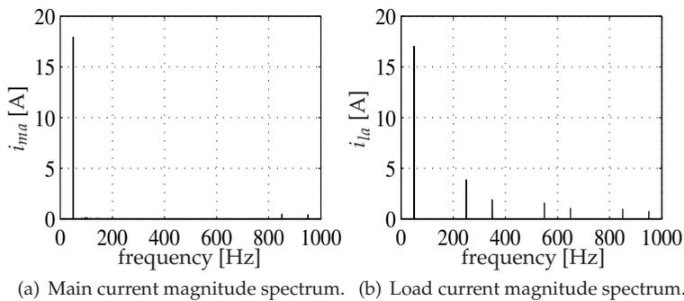
(a) Main current magnitude spectrum. (b) Load current magnitude spectrum.
