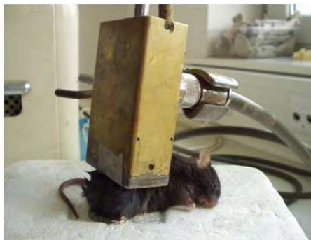
Fig. 19. Waveguide applicator for biological experiments
