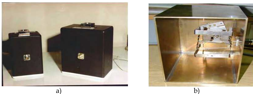
Fig. 2. a) Dielectric filled waveguide applicator, b) air filled Evanescent mode applicator.
