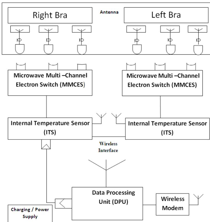
Fig. 5. The functional scheme of Multi-Channel Microwave Radiometer
