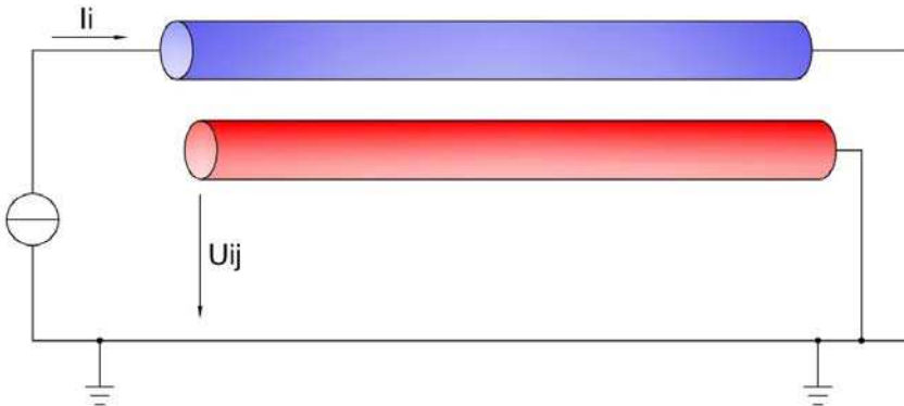
Fig. 5. Mutual impedance calculation
