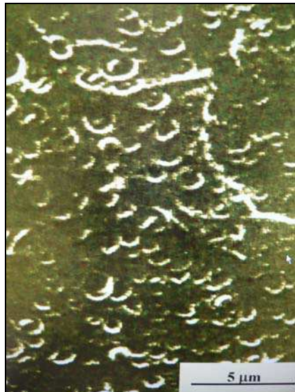
Fig. 3. Surface of COC-blend with designed pores with diameters ranging from 0.6 to 1.5 \mu\text{m} In order to improve the bonding between the polymer blend and collagen, the surface of the polymer matrix was modified by the action of a nitrogen and/or oxygen microwave plasma. The plasmatic modification resulted in a significant increase of surface hydrophilicity demonstrated by a decrease of water contact angle.
