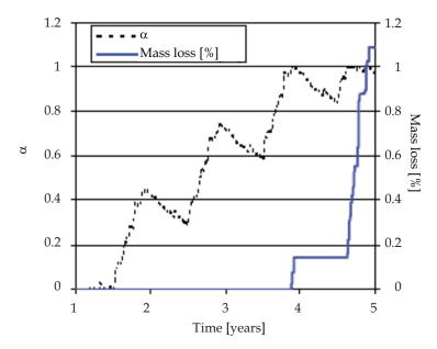
Fig. 6. No activation of growth or decay development during the first and second years, an activation of decay process after 4 years exposure may be expected (Viitanen et al 2010b)
