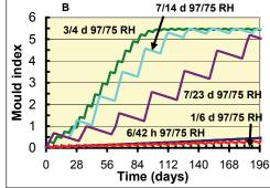
Fig. 2. Modelling the effect of varied fluctuating humidity conditions on the development of mould index in pine sapwood (Viitanen et al. 2000)
