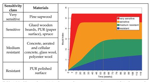
Table 4. Mould growth sensitivity classes and some corresponding materials in the research. The figure in table illustrates the predicted mould growth for the established sensitivity classes for constant conditions at 97 % RH and 22 C (Viitanen et al 2011)
