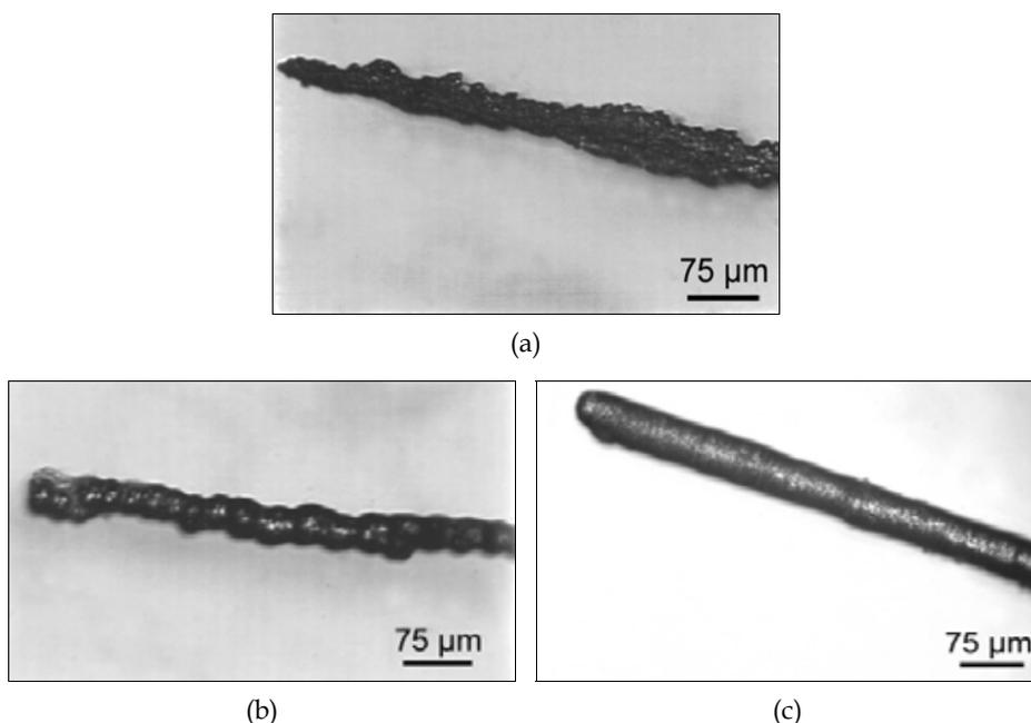
Fig. 2. Optical micrographs (OM) of the nickel micrometer columns fabricated by the MAGE process in a sulfate bath where the initial gap between the electrodes was the same (at  $10 \mu\text{m}$ ) but their dc-voltage bias and the motion mode of the microanode changed as follows: (a) bias at 5.0 V and the microanode moved continuously at a rate of  $1.8 \mu\text{m s}^{-1}$ , (b) bias at 5.0 V and the microanode moved intermittently and (c) bias at 3.5 V and the microanode moved intermittently
