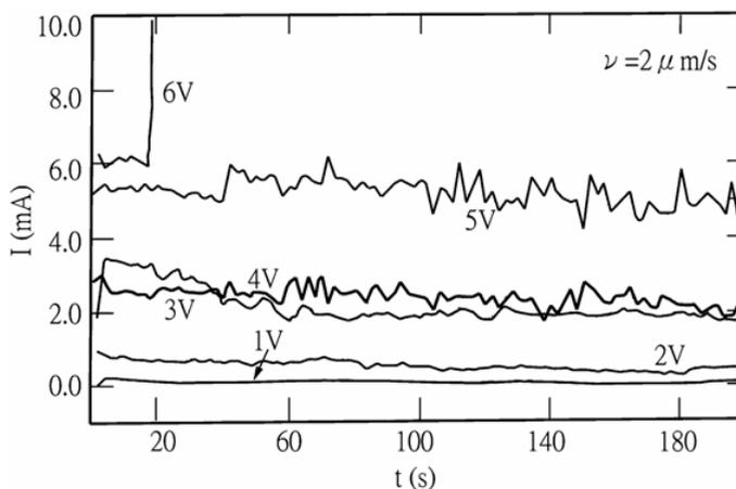
Fig. 4. A plot of current against the electroplating time for the MAGE process conducted at various biases and the microanode moved continuously at a constant rate (e.g.,  $2.0 \mu\text{m s}^{-1}$ ). The initial gap between the microanode and the Cu-substrate was  $20 \mu\text{m}$
