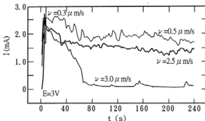
Fig. 5. Current against the electroplating time in the process of continuous MAGE at a bias of 3.0 V with the motion rate of the microanode varying in the range from 0.3 to  $3.0 \mu\text{m s}^{-1}$ . The initial gap between the microanode and the Cu-substrate was  $20 \mu\text{m}$
