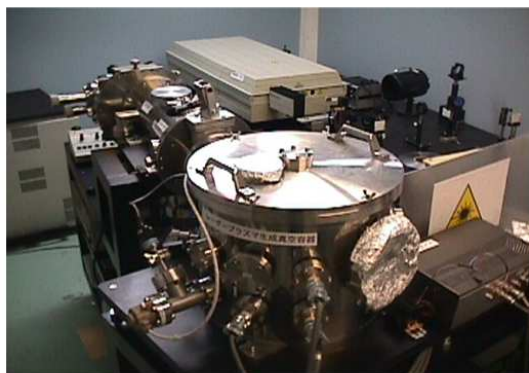
A reflectance measurement tool by laser plasma EUV light source
