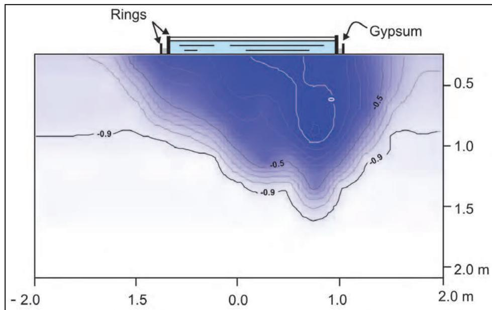
Fig. 7. Best selected model simulation output in order to fit the shape of the wetting front at  $t = 80 \text{ min}$ . Contour lines represent model output expressed as matric potential (m) in the fracture.
