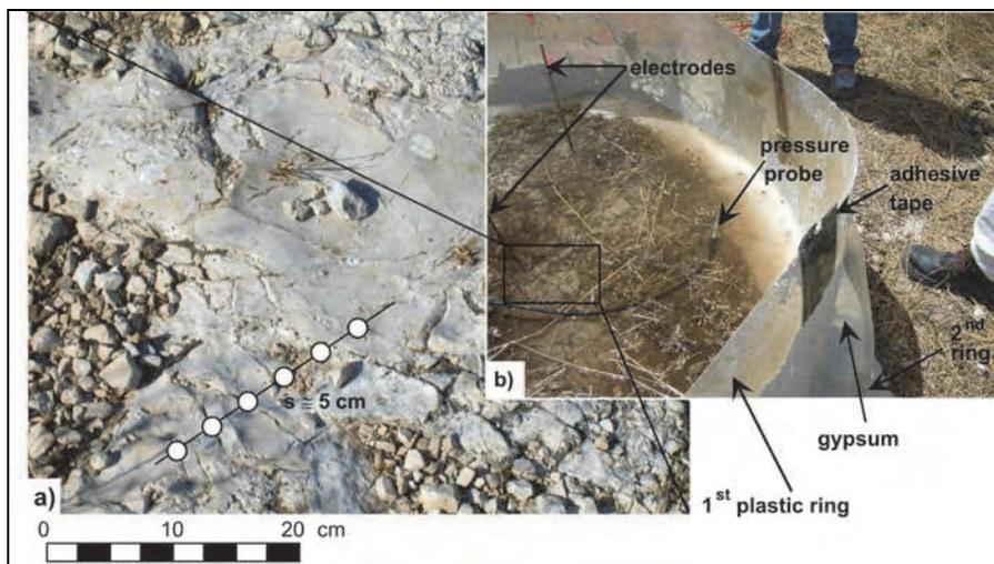
Fig. 2. Test # 1 at the Altamura site: a) fractured limestone with visible fractures of about 5 cm of spacing ( $s$ ); b) plastic ring infiltrometer resting directly on the ground and sealed with gypsum by using a second ring.
