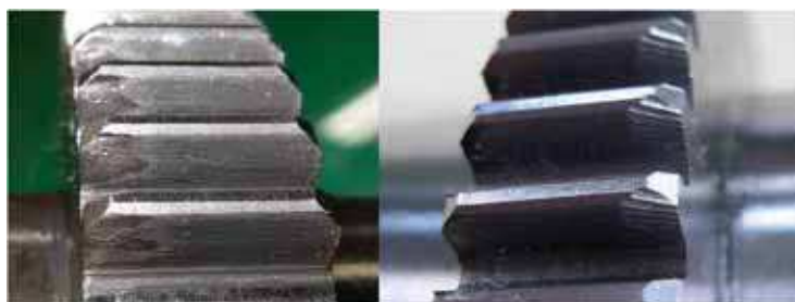
Fig. 8. Gear tooth worn by misalignment
