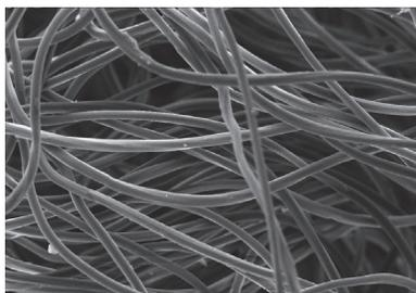
Fig. 1. Scanning electron micrograph (SEM) image of nanofibers.
