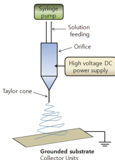
Fig. 2. Schematic image of the electrospinning method.
