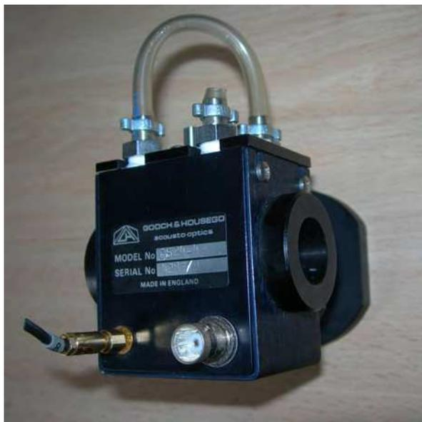
Fig. 16. AOD used for experimental verification
