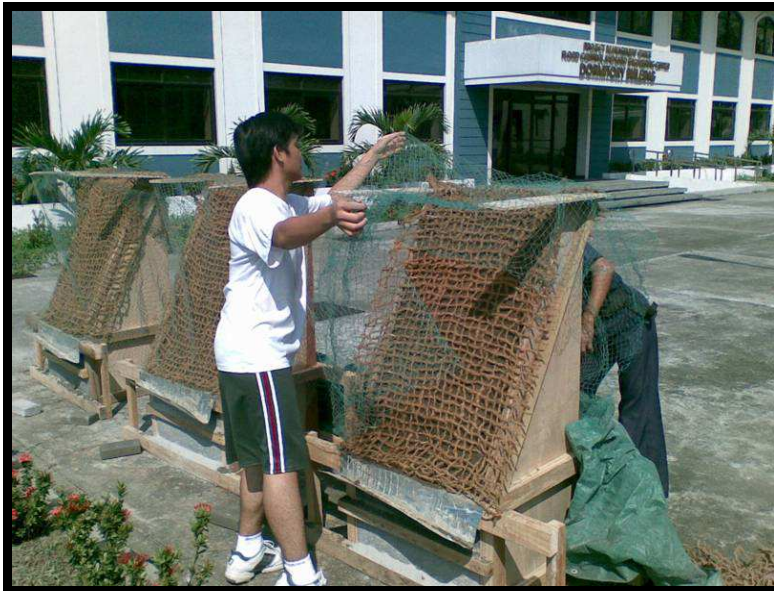
Fig. 5. Hydroseeded test boxes covered with coconet. The green net is used for protection from birds and other factors.
