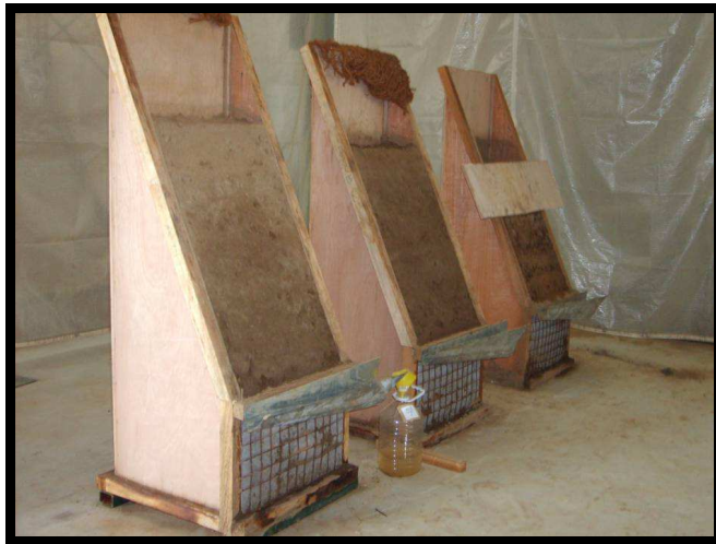
Fig. 2. Test boxes shown with compacted soil.
