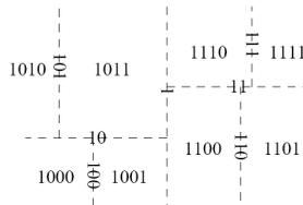
Fig. 1. Indexing scheme for two-dimensional  $kd$ -tree.
