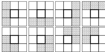
Fig. 9. Filters with size  $3 \times 3$  for detecting whether a background pixel is beyond the projected silhouette of the object. If one of the eight masks matches the neighborhood of a background fragment, it is not filled. White cells indicate background pixels, dark cells may be background or non-background pixels.
