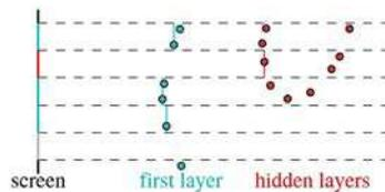
Fig. 11. Depth peeling for point cloud surfaces.
