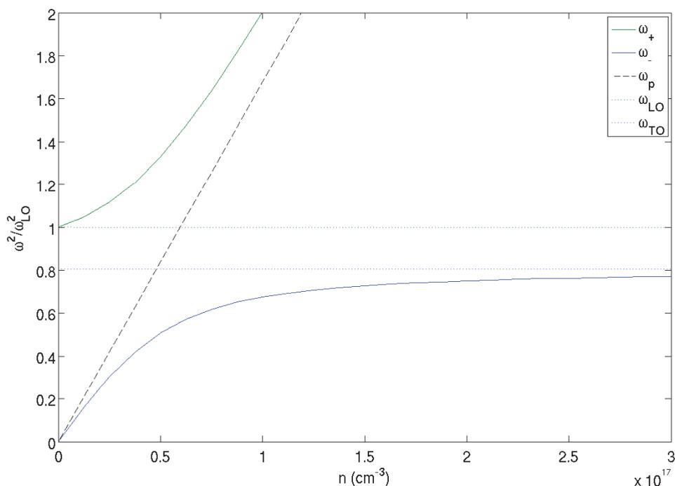
Fig. 3. A plot of the frequencies associated with the hybrid modes. Calculations done for Cd<sub>0.28</sub>Hg<sub>0.72</sub>Te at 300 K. The band gap is 0.271 eV.
