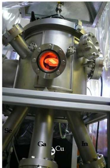
Fig. 8. Thermal co-evaporation system with Knudsen effusion cells to deposit Cu(In,Ga)Se<sub>2</sub> thin films
