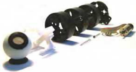
Fig. 16. The body of the MAC-EYE robot. All the motors are integrated within the body; furthermore, all the cables from and to the eye-ball and the embedded optical tension sensors are routed inside of the structure.
