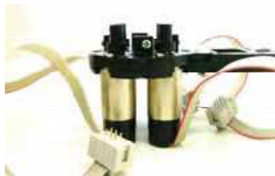
Fig. 15. Four DC motor actuate the tendons; pulleys route the tendons towards the eye-ball
