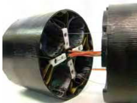
Fig. 17. Implementation of the embedded sensors for measuring the mechanical tension of the tendons. The picture shows the shutter and its preloading spring, cables and tendons.
