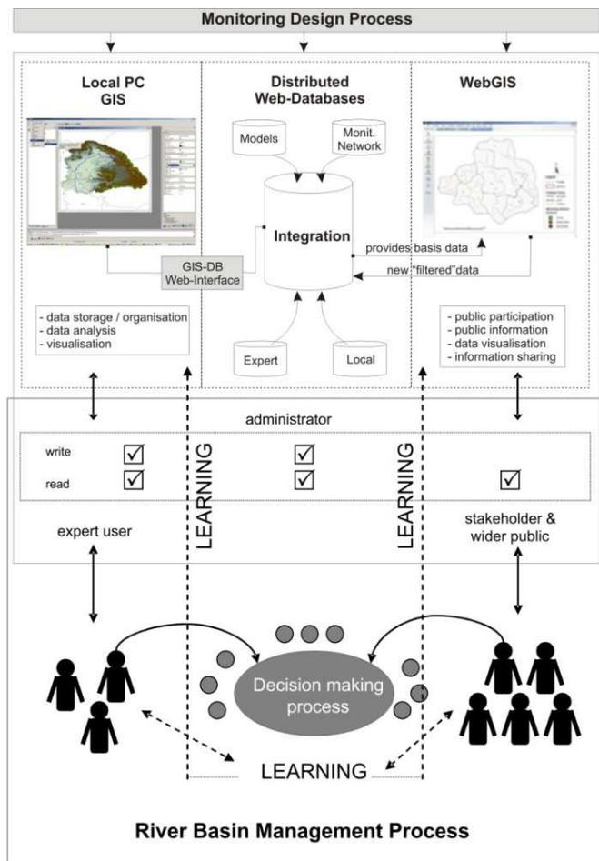
Fig. 2. Technical components of AMIS.
