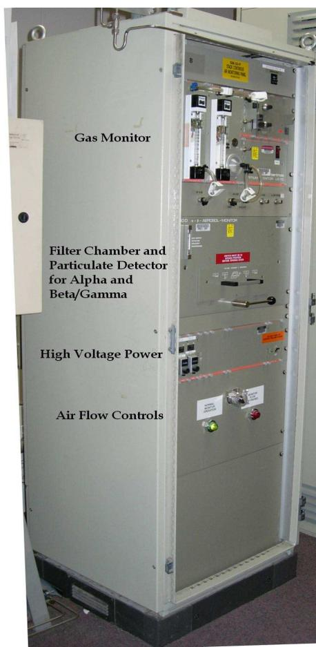
Fig. 4. Combination continuous air monitor for particulates and gases
