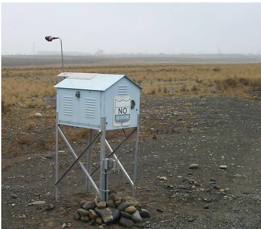
Fig. 5. Environmental air monitoring station
