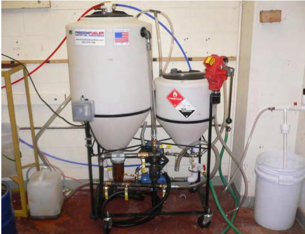
Fig. 3. Biodiesel Processor with a capacity of 40 gallons/day
