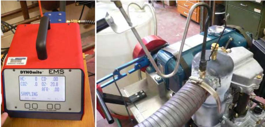
Fig. 9. Gas Analyzer and emission probe
