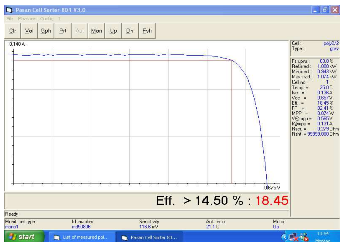
Fig. 8. Experimental I-V curve of the solar cell performed with the Pasan machine.
