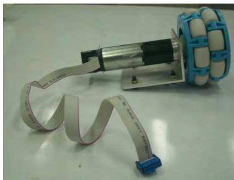
Fig. 7. An omni-directional wheel was driven by DC servo motor
