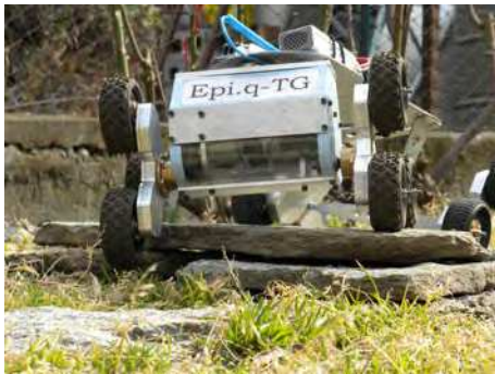
Fig. 17. Epi.q-2 traversing an obstacle, on uneven ground
