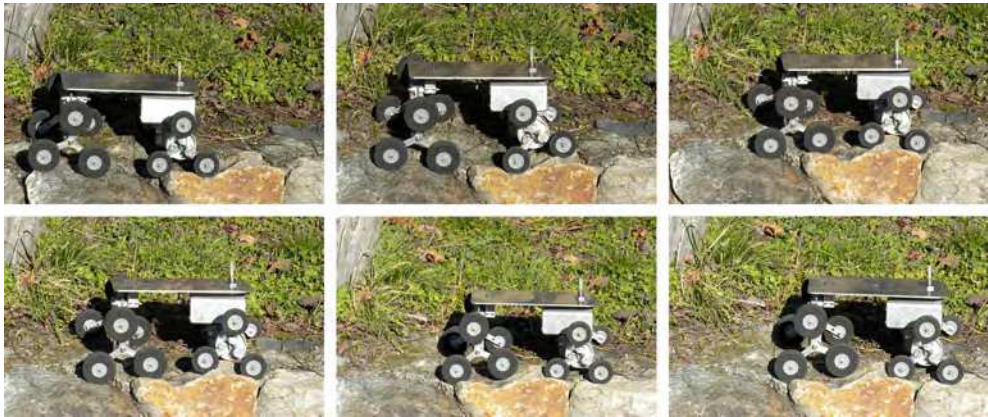
Fig. 12. Epi.q-1 in advancing mode, on uneven ground
