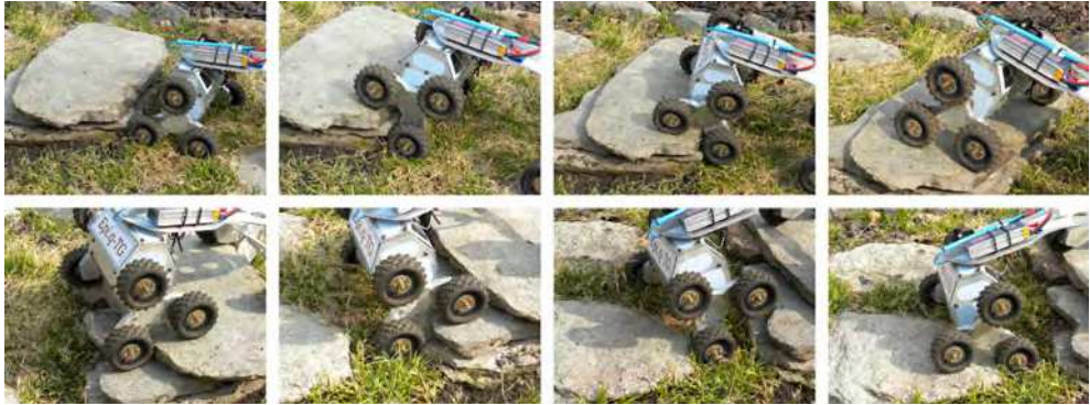
Fig. 13. Epi.q-2 negotiating an obstacle
