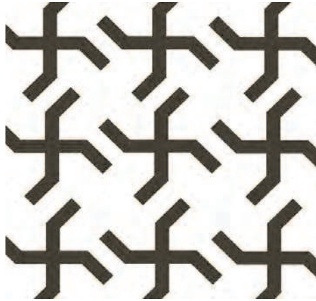
Fig. 4. Planar chiral structure made by arrays of gammadians arranged in two-dimensional square gratins (Papakostas et al., 2003).
