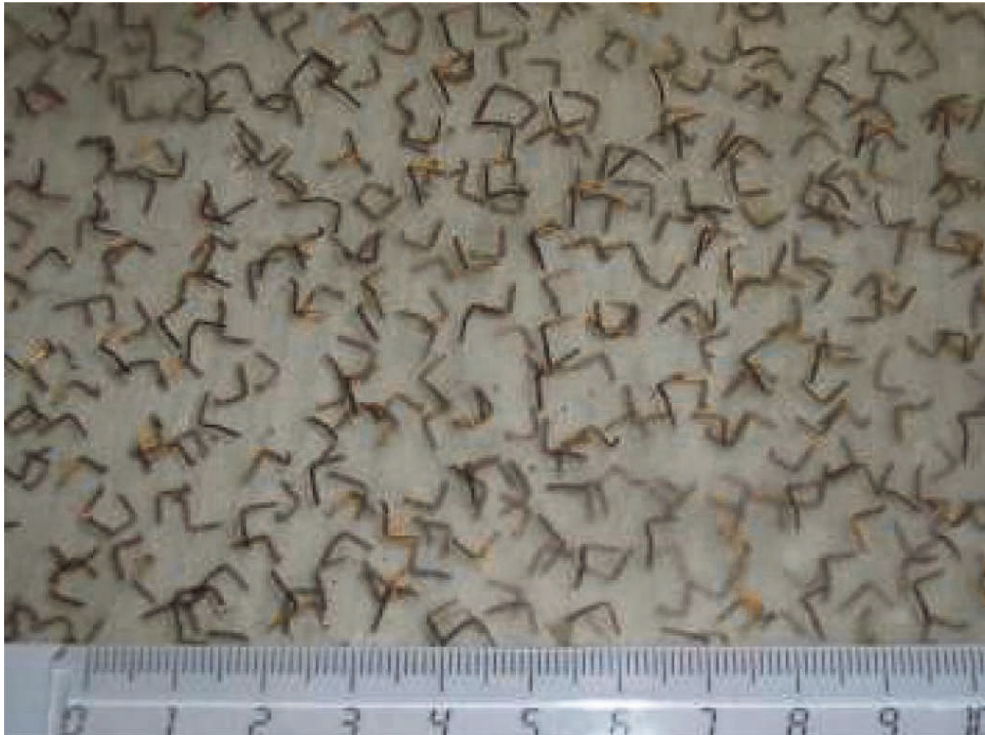
Fig. 2. Crank-based artificial chiral material. Chiral elements were produced from a 0.4 mm diameter and 12.6 mm length copper wire by bending in three segments by two 90 angles, all with the same handedness. The elements were dispersed in an epoxy resin with a low curing temperature (Molina-Cuberos et al., 2009).
