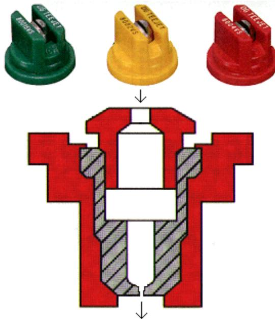
Fig. 9. Low drift nozzles (Spraying Systems Co.)
