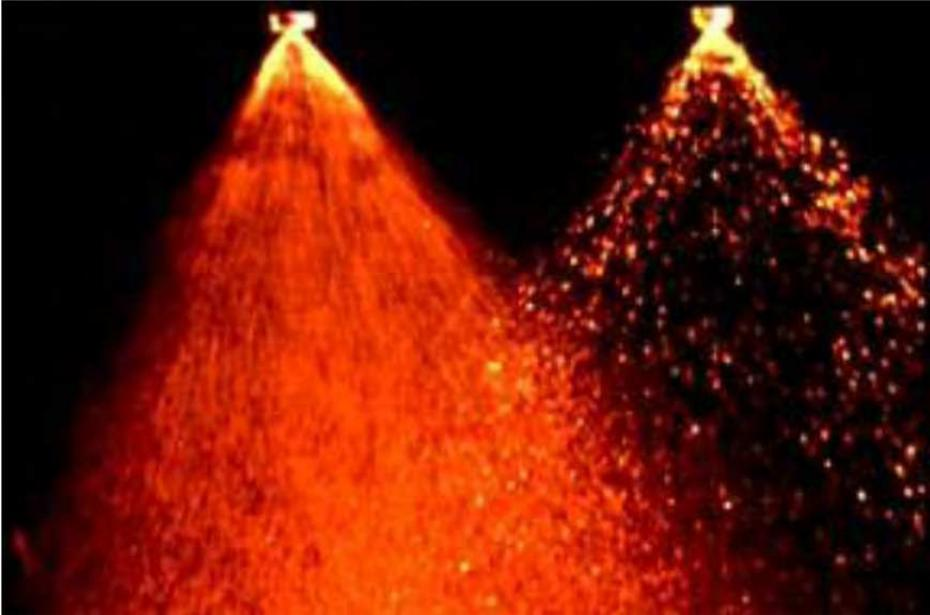
Fig. 1. Effects of nozzle type on the droplet size
