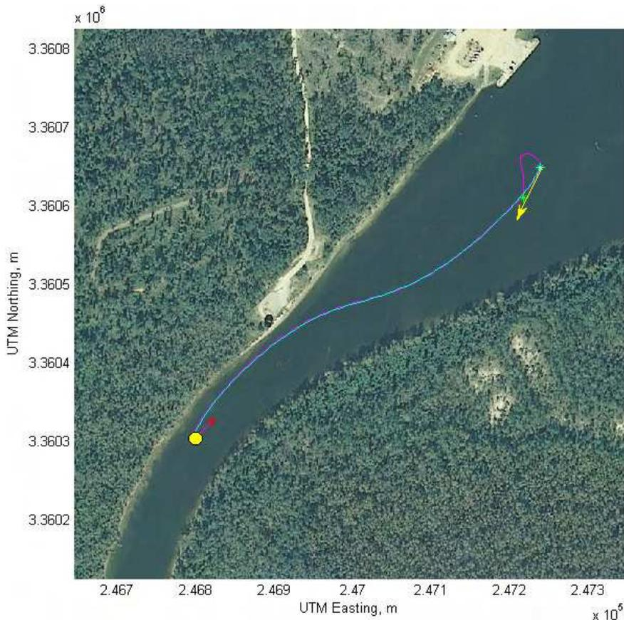
Fig. 27. Path-following controller test on the Pearl River
