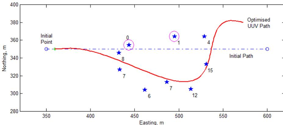
Fig. 23. Simulation results for a feature-based navigation application
