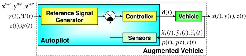
Fig. 1. A. UUV augmented with an autopilot
