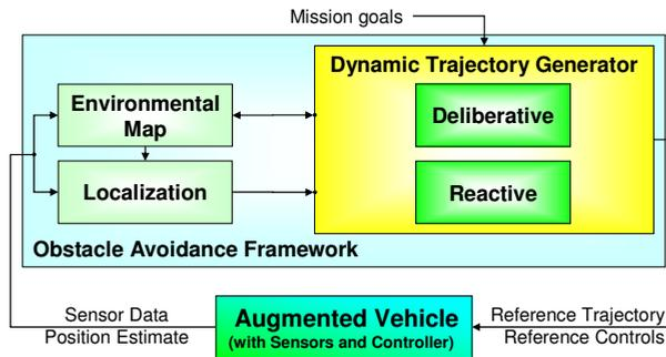
Fig. 13. Components of the NPS OA framework
