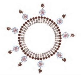
Fig. 8. Depicts a unique microbubble construct for gene delivery. The parent microbubble is PEG'ylated but the DNA (or siRNA) is condensed into nanoparticles that are bound to the surface of the microbubble. The nanoparticles have targeting ligands to bind to cell specific epitopes. Note also that the construct could be modified to comprise endothelial targeting moieties on the microbubble so that the microbubble could bind to endothelial epitopes.
