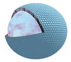
Fig. 1. Depicts a microbubble coated with a film of stabilizing material.
