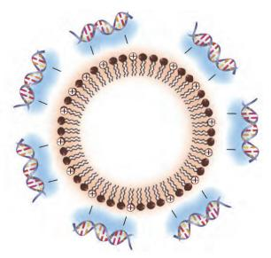
Fig. 4. Depicts a microbubble for gene delivery. The gaseous core is coated by a monolayer of phospholipid containing cationic lipid imparting a net positive charge to the microbubble. DNA, as a polyanion, is adsorbed electrostatically to the exterior surface of the microbubble.
