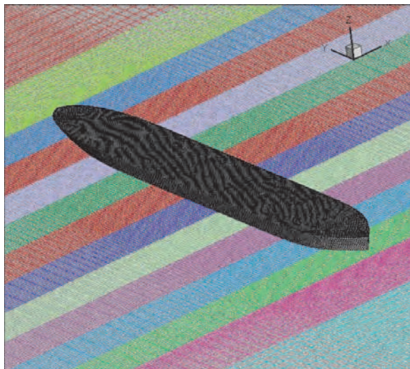
Fig. 6. Grid generated around the Series-60 hull (top view).
