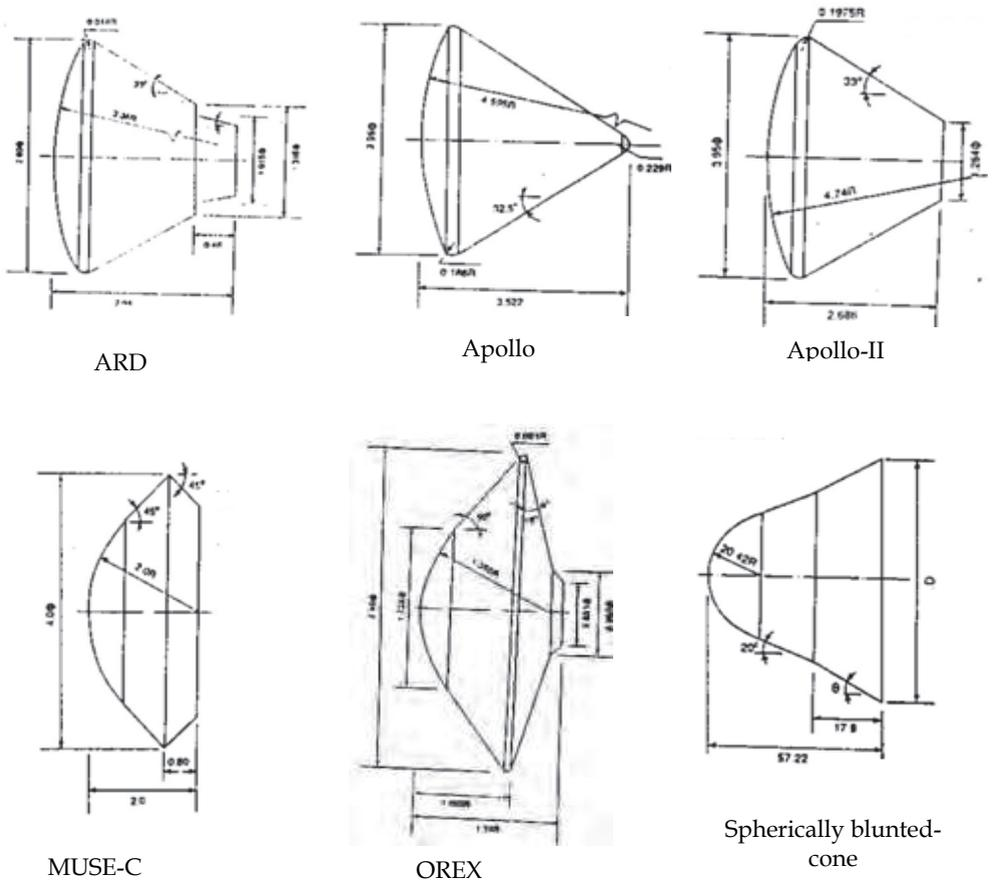
Fig. 2. Geometrical details of various reentry capsules.
