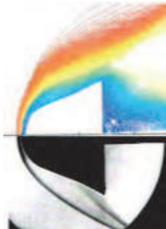
Fig. 4. Comparison between density contour and schlieren picture.
