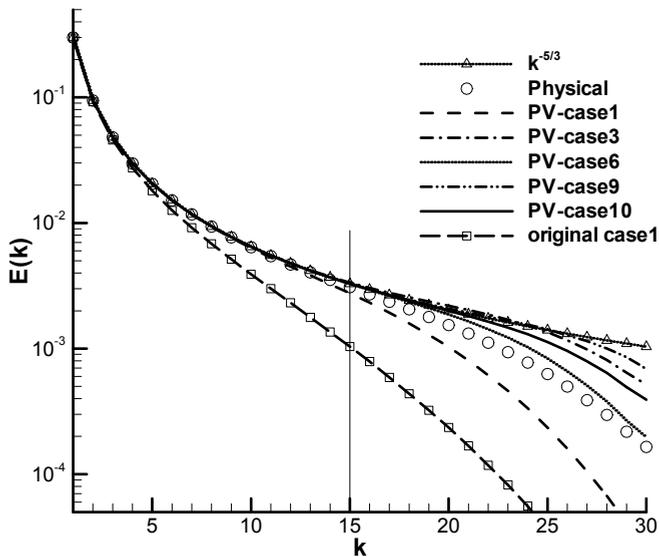
Fig. 4.13. Effect of the PV-filters on the  $k^{-5/3}$  spectrum.
