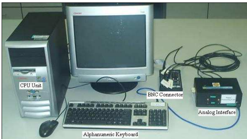
Fig. 3. PBAS system components.
