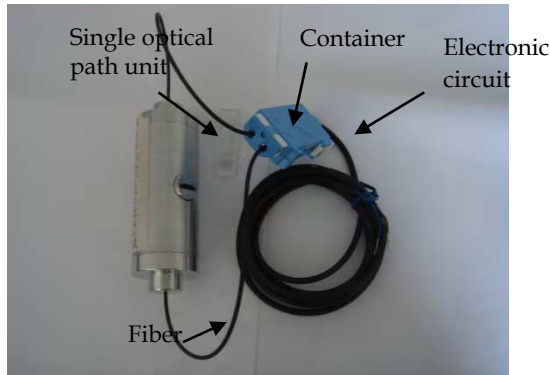
Fig. 19. Prototype of the single optical path absorbance biometric system.
