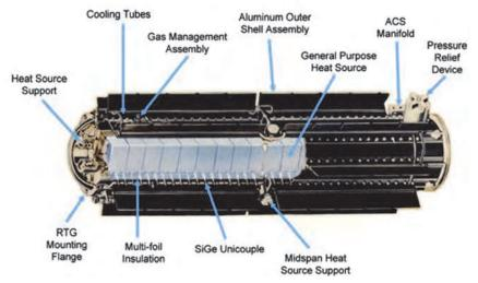
Fig. 3. Radioisotope Thermoelectric generator (RTG). (Source NASA/DOE/JPL)
