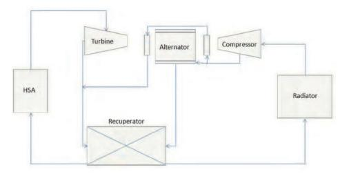
Fig. 5. Dynamic Isotope Power System Cycle
