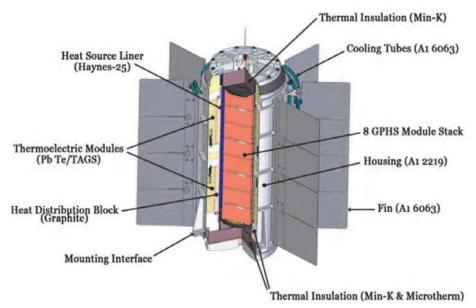
Fig. 4. Multi-mission Radioisotope Thermoelectric Generator (MMRTG). (Source NASA/DOE/JPL)
