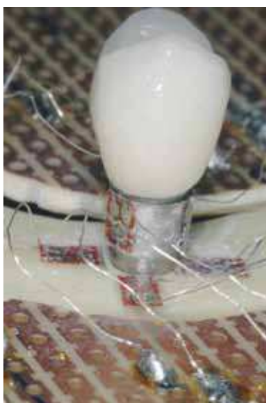
Fig. 8. A bone simulated model was used to quantify the tension around the cervical area of the implant when the restoration is connected.
