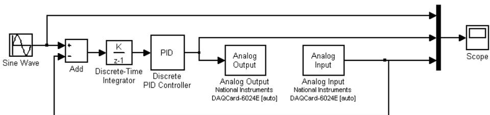
Fig. 2. Simulink model for the RTWT application
