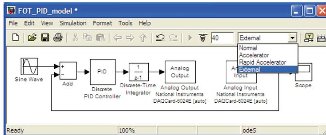
Fig. 5. Configuring the simulation in External mode
