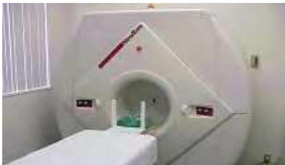
Fig. 5. Cone-beam computerized tomography (CBCT) device (NewTom)
