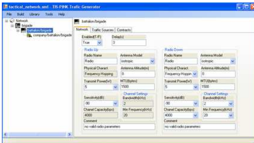
Fig. 3. TPGen application, where tree-view is visible in the left panel and network editor on the right panel.
