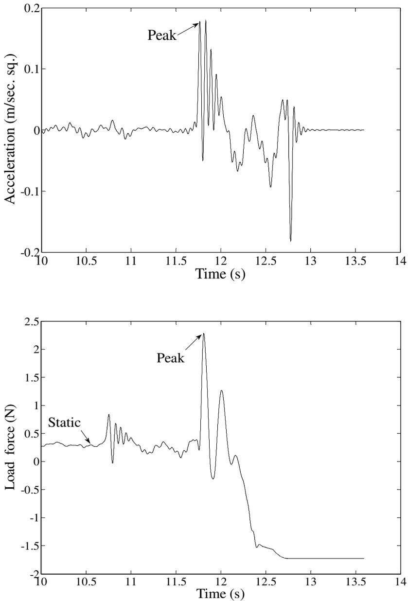
Fig. 9. Time trajectories of displacement , velocity , acceleration and load force for a trial when a subject manipulated the small size PAO with the system at condition 1 ( $m_1=0.5\text{kg}$ ,  $m_2=0.03\text{kg}$ ).
