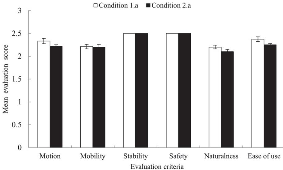
Fig. 12. Mean performance evaluation scores for small size object for condition 1.a ( $m_1=6 * e^{-6t} + 0.5, m_2=0.03$ ) and condition 2.a ( $m_1=6 * e^{-6t} + 1.0, m_2=0.03$ ) after the control modification.
