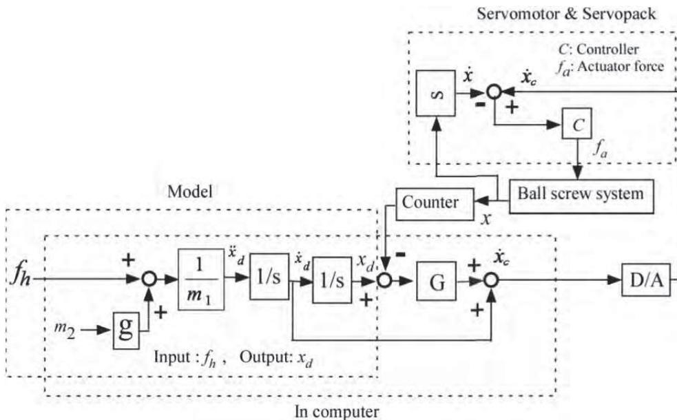
Fig. 5. Block diagram of the power-assist control, where  $G$  denotes feedback gain, D/A indicates D/A converter and  $x$  denotes actual displacement. Feedback position control is used with the servomotor in velocity control mode.
