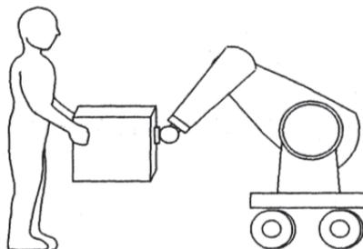
Fig. 1. A human manipulates (lifts) an object with a power assist robot and feels a scaled-down portion of the weight.
