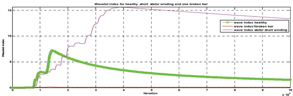
Fig. 14. Wavelet index for fault detection
