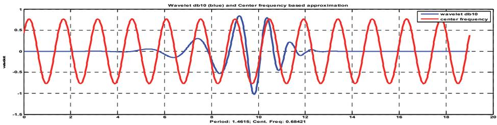
Fig. 8. Daubechies wavelet (db10) and central frequency
