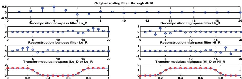
Fig. 6. Wavelet decomposition and reconsstrction f filters
