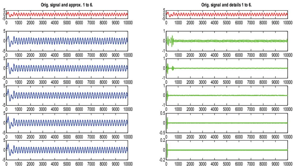
Fig. 11. Approximation and details signal in healthy motor
