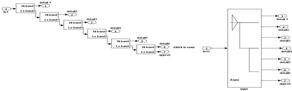
Fig. 7. DWT filters and levels using simulink
