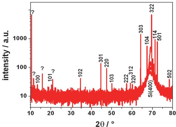
Fig. 2. The typical XRD-SR pattern of nanocomposite  $\text{SiC}_x\text{N}_y$  film shows that the peaks' position is close to standard  $\alpha\text{-Si}_3\text{N}_4$  phase. There are some unknown peaks at small diffraction angles indicated by "?", which do not correspond to peaks positions of other known phases of the Si-C-N system.
