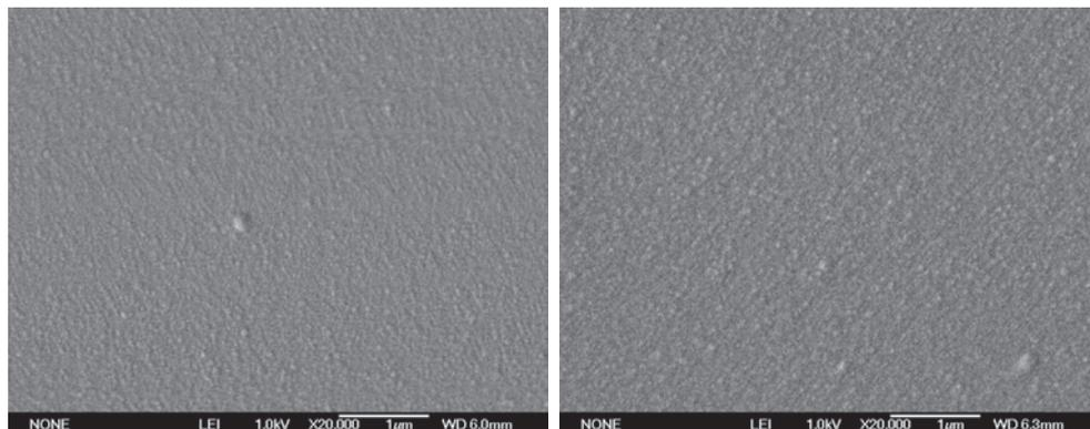
Fig. 1. Typical SEM images of surfaces of PECVD SiC<sub>x</sub>N<sub>y</sub> film (left) and BC<sub>x</sub>N<sub>y</sub> (right).
