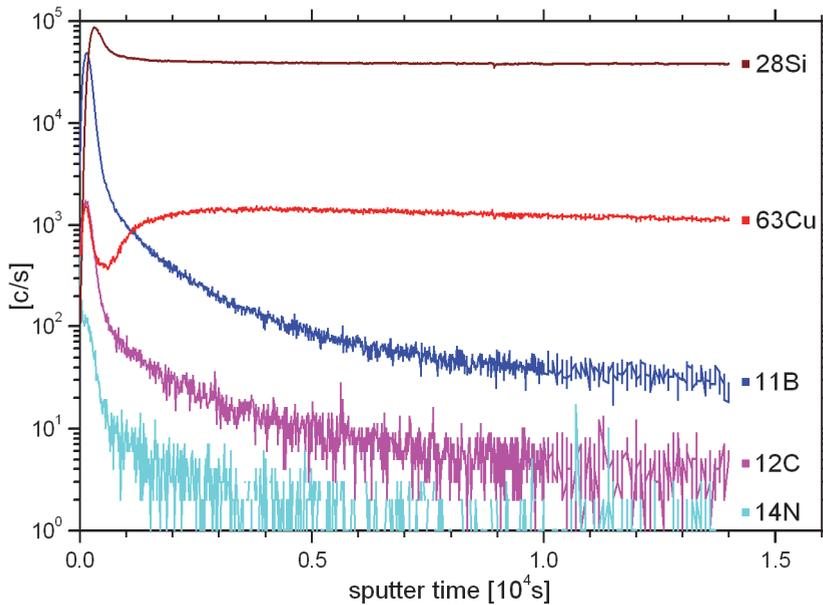
Fig. 8. SIMS profile of a layered system BCN/Cu/Si.
