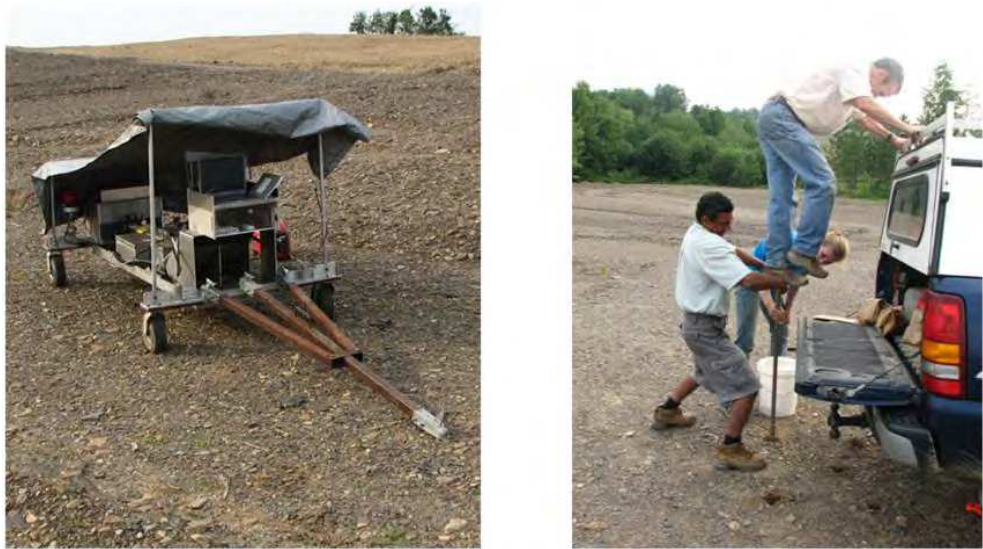
Fig. 14. Comparison of sampling abandoned minefield restored with its original overburden using the INS system on the left, and an attempt using conventional coring on the right, many cores could not be sampled deeper than 10 cm.
