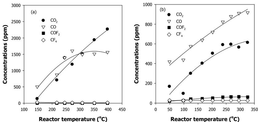
Fig. 13. Byproducts distribution: (a) with alumina and (b) with zirconia ( $C_2H_2F_4$ : 2,000 ppm;  $O_2$ : 2.0% (v/v); input power: 60 W)
