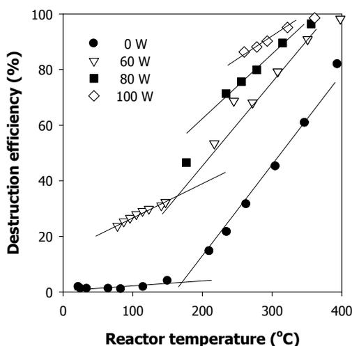
Fig. 8. Comparison of  $\text{C}_2\text{H}_2\text{F}_4$  destruction efficiencies between catalysis alone and plasma-catalysis over a temperature range up to 400°C ( $\text{C}_2\text{H}_2\text{F}_4$ : 2,000 ppm;  $\text{O}_2$ : 2.0% (v/v))
