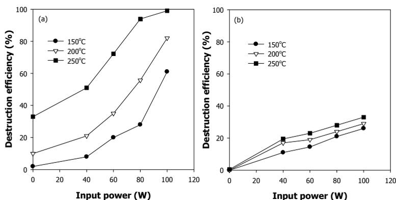
Fig. 15. Effect of the electric power on the decomposition of  $\text{CHF}_3$  (a) with alumina and (b) with glass beads ( $\text{CHF}_3$ : 2,000 ppm;  $\text{O}_2$ : 1.0% (v/v))
