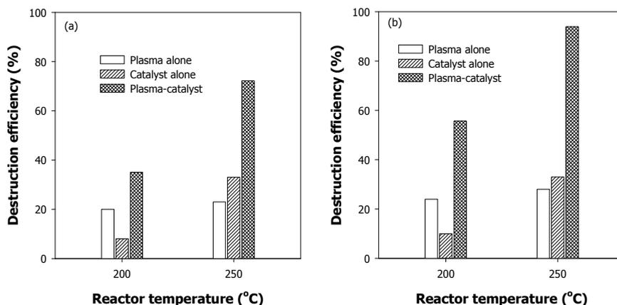
Fig. 14. Comparison of decomposition efficiency between the plasma alone, the catalyst alone and the plasma-catalyst combination at input powers of (a) 60 W and (b) 80 W ( $CHF_3$ : 2,000 ppm;  $O_2$ : 1.0% (v/v)).
