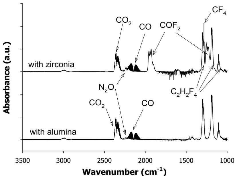
Fig. 12. FTIR spectra of the gas processed in the plasma reactor ( $C_2H_2F_4$ : 2,000 ppm;  $O_2$ : 2.0%(v/v); input power: 60 W)
