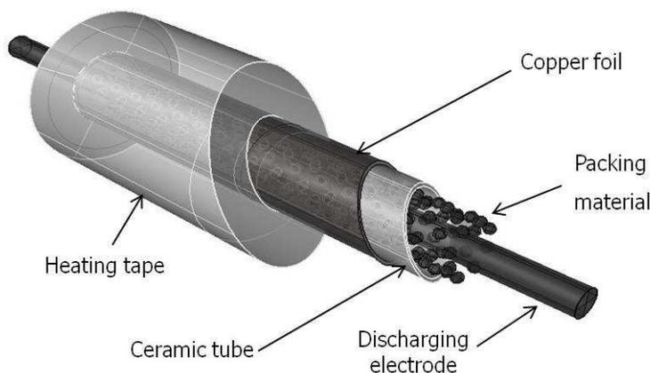
Fig. 3. Schematic diagram of the nonthermal plasma reactor
