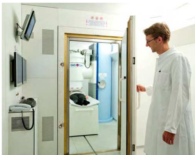
Fig. 3. Apollo CXS system: view from the preparation room into the acquisition room soon before the acquisition is carried out. The patient lies on the bed as close as possible under the dewar bottom.
