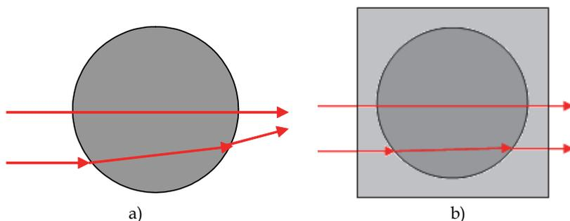
Fig. 3. Illustration of the laser path problem in optical CT: a) bending of the laser path because of the refraction at the surface of the cylindrical dosimeter; b) the use of refractive index matching liquid to maintain straight line laser passage.
