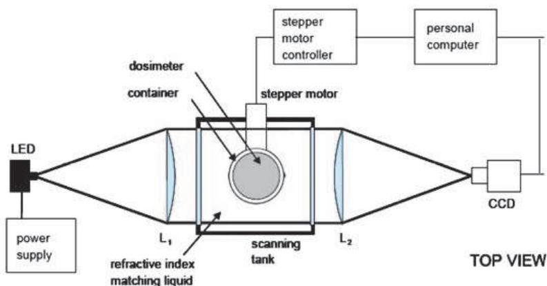
Fig. 2. Schematic diagram of a CCD-camera based optical tomography scanner.
