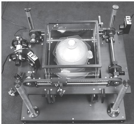
Fig. 1. Top view of the OCT-OPUST<sup>TM</sup> research scanner (MGS Research, Inc., Madison, CT, USA) with a Barex gel cylinder mounted in the scanning tank.
