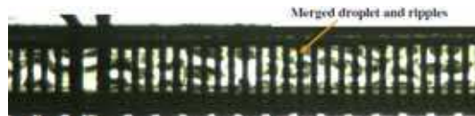
Fig. 27. A drop-wise slug flow pattern in a hydrophobic microchannel (Choi & Kim, 2008)
