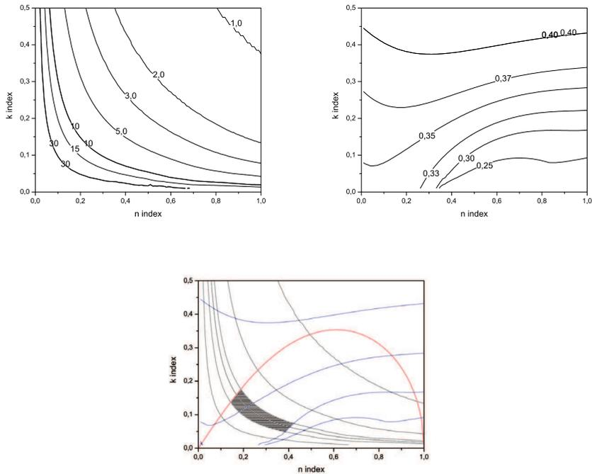
Fig. 2. (top left) Critical fluence  $F_c$  in  $J.cm^{-2}$  as a function of  $n$  and  $k$  for  $\tau = 3 ns$ . (top right) Scaling law exponent  $x$  as a function of  $n$  and  $k$  for  $\tau \in [1 ns; 10 ns]$ . (bottom) Intersection of (a) and (b), the highlighted area delimits the region satisfying experimental data.
