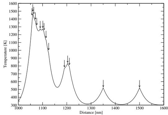
Fig. 3. Spatial temperature evolution resulting from a particular random throwing. 15 ADNS are present,  $A/\rho C = 10^{13} K.s^{-1}$  and  $\tau = 1 ns$  are used. The temperature rise is enhanced when several ADNS aggregate. Defects positions are shown by vertical arrows.
