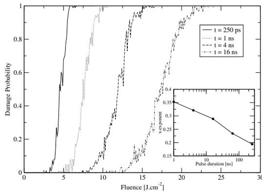
Fig. 4. Evolution of the damage probability as a function of fluence within the 1D model. Four pulse durations are considered :  $\tau = 250ps, 1ns, 4ns$  and  $16ns$ . Parameters are  $n_{ADNS} = 100$  and  $N = 10000$ . 200 drawings have been performed for each fluence. Sub-figure displays the scaling law exponent as a function of the pulse duration (see text).
