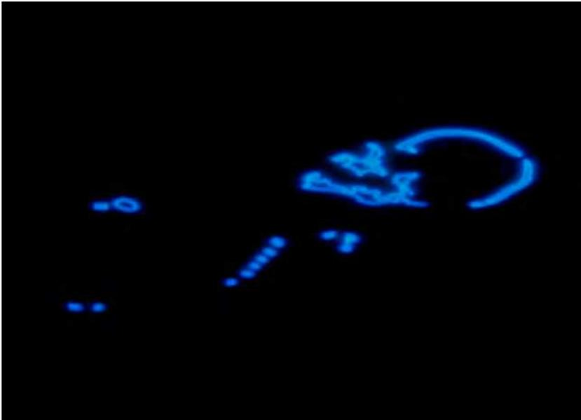
Fig. K. Slice showing the laser beam during the hardening process of the photo sensible resin on SLA VIPER Si
