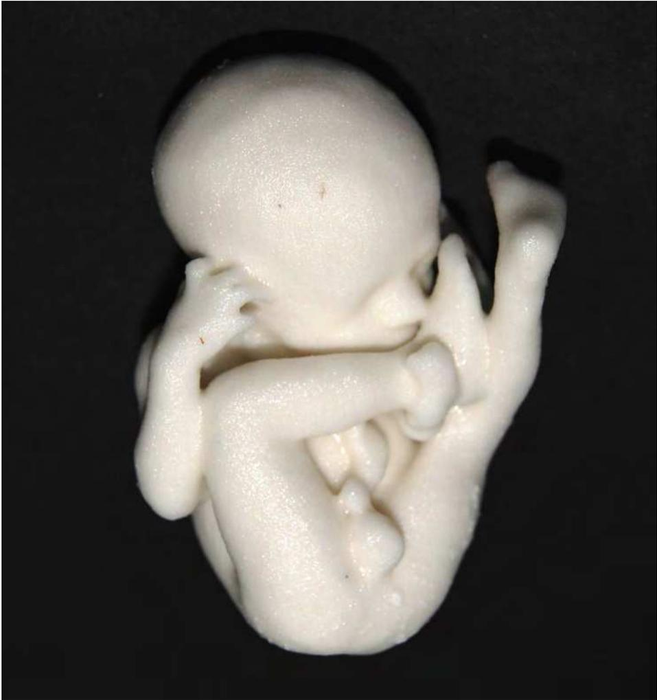
Fig. F. 26 weeks physical model of fetus built in Z Corp 510 from Ultrasonography 3D files.
