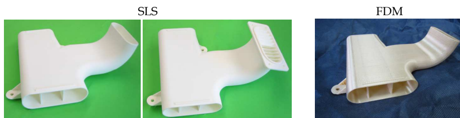
Fig. 9. AMT manufactured air ducts
