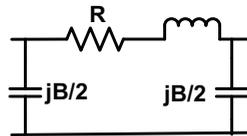
Fig. 5. Equivalent circuit for lines and cables
